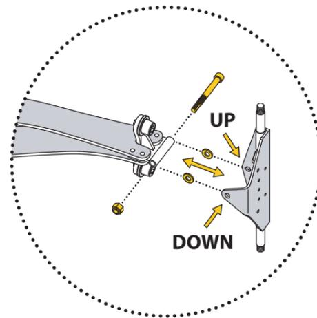
Take the truck and mount it on the frame. Place the bolt and the washers, as shown. Both washers should be on the inner side of the truck. Tighten the nut well and make sure the truck can pivot freely. If it doesn't, slightly loosen the nut with a quarter revolution.
