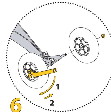
Place the rear wheels onto the axles, make sure all 4 bearings are in place, and screw the nuts. Tighten carefully, as overdoing it can lock the bearings, thus preventing the wheels' free rotation. We suggest that you tighten the nut well at first - until it starts to block the wheel (1), and then make a quarter revolution backwards to loosen it slightly (2).
